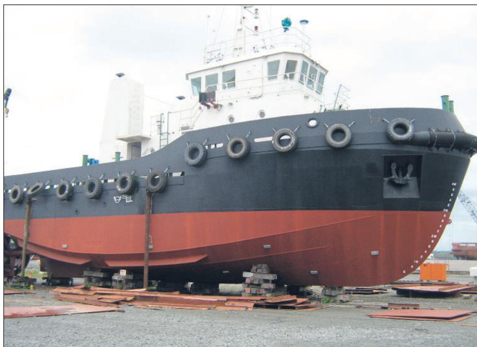
A twin screw, 30-metre, 2 x 1200 horse power Cummins NKK class
